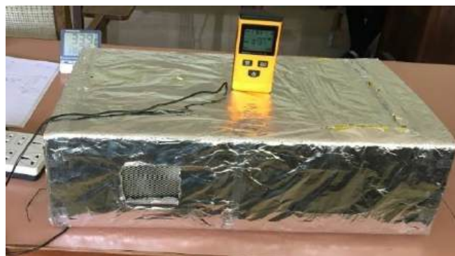
Figure 5: The EMFr detector that is equipped on the treatment chamber.
